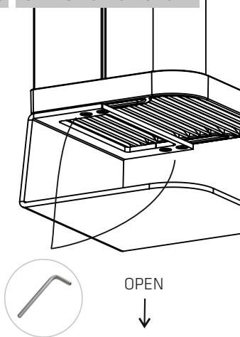
2D **CHANGING A UV-C TUBE**
