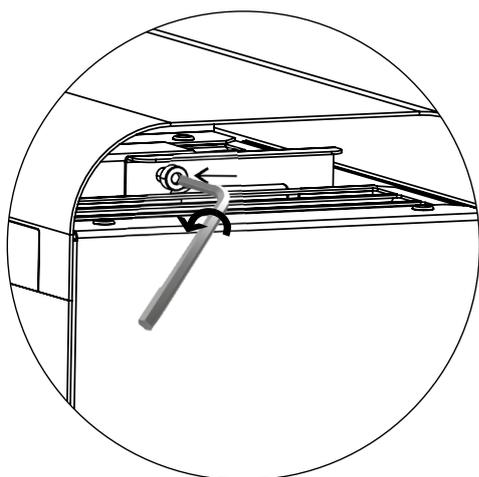
To ensure a higher degree of safety against exposure to UV-C radiation, we offer additional protection that prevents the luminaire cover from being opened.
